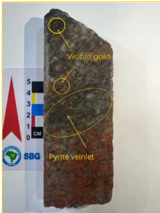
Visible gold in silicified veinlets cross-cutting perthitic granite in hole 22ZS_014.
